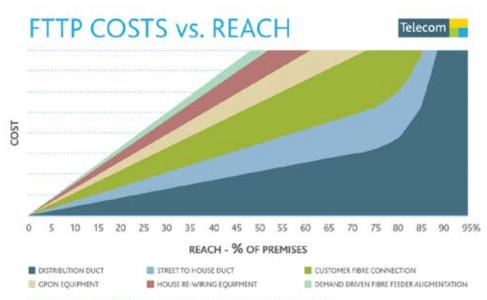
NOTE : MODELLED ON USE OF TELECOM NETWORK AND DEPLOYMENT TO ONE SIDE OF STREET
